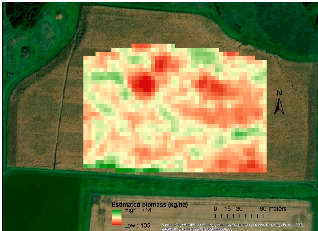
Figure 5. Spatial variability in maize biomass at the five leaf collar stage estimated using NDVI values from RapidEye satellite imagery.
